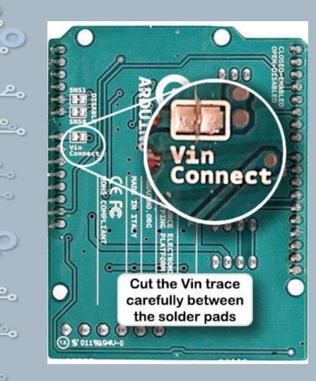
Cut the Motor Shield Vin connecting trace.
